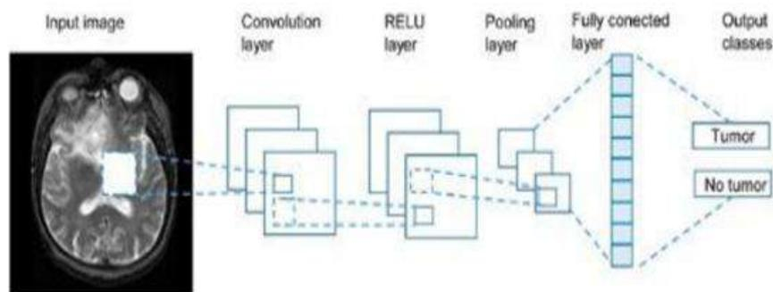
**Figure 1:** Convolutional Neural Network work
