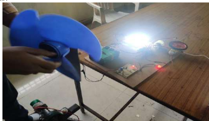
Figure 5: Working Prototype System with Plastic fan as a Source of Power Generation
