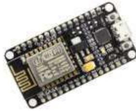
**Fig:** NodeMCU Development Board
