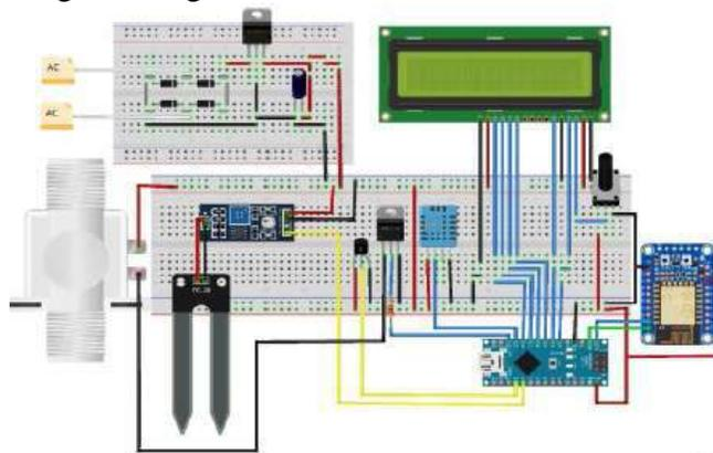
Fig.5 Integration of the full circuit
