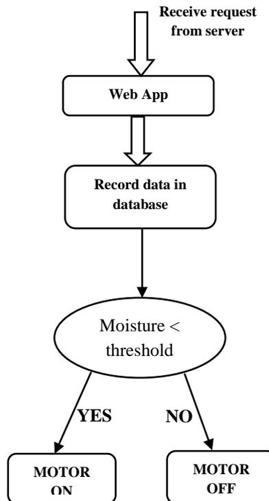
Fig. 3 Process flow for irrigation
